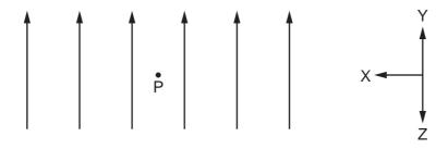
The field lines (lines of force) are evenly spaced and parallel.
